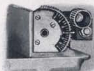
End view of fence tilting device shows pinion and rack tilt mechanism. Accurate gauge shows angle of tilt.
