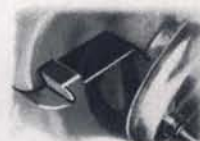
View showing expensive dovetailed ways holding table in position. Adjustable gibbs take out any play.
