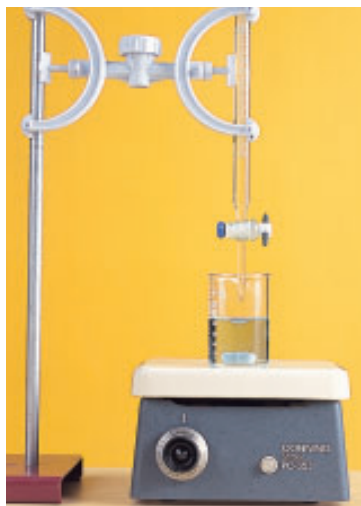
Figure 4 A burette and magnetic stirrer provide for a very efficient procedure.
