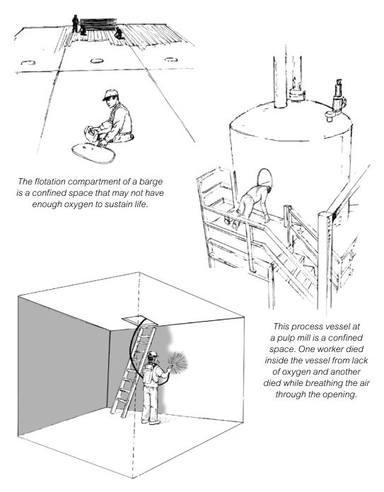
This water cistern is a confined space with limited access and ventilation. While a waterproof coating was being applied, flammable vapours were generated. The vapours ignited, causing an explosion.
