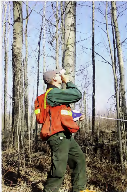
Forester Dennis Froese using clinometer to measure height of tree for timber cruise, East Peace Area, 2004
