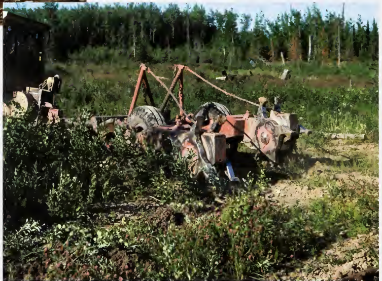
Bracke scarifier, one of the many mechanical tools used to expose mineral soil during site preparation, readying a site for planting Alberta Government, AFHPC
