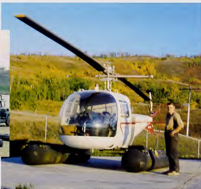
Exchanging skids for floats on a Bell 47J, mid-1960s Cliff Smith
