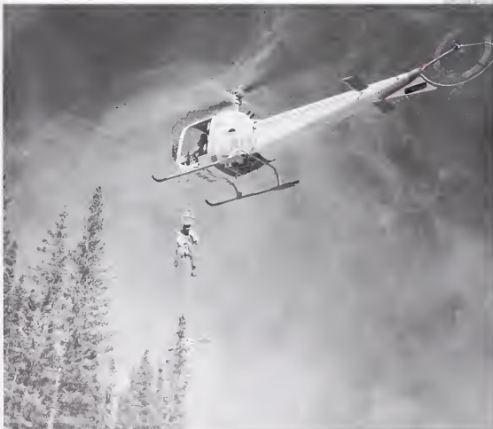
Rangers being trained for lowering to the ground by sky-genie, a winch attached to a helicopter. The rangers were able to clear landing pads in forested areas for helicopter access – tower or lookout sites, fires, etc. Ranger has a power saw attached on a rope. Helicopter used in this training is the Alberta Forest Service Bell 47AJ, CF-AFK, early 1960s Alberta Government, AFHPC
