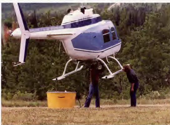
Hooking up the Water Buoy water bucket to the cargo hook and attaching the electrical cord on Bell 206 Jet Ranger JEL, Kananaskis Ranger Station, Canmore District, Bow Crow Forest, spring, 1981
