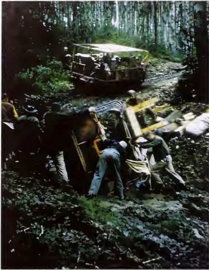
Forest survey crew trying to upright a rolled Bombi, 1959. A Bombi was a tracked personnel carrier made by Bombardier Cliff Smith
