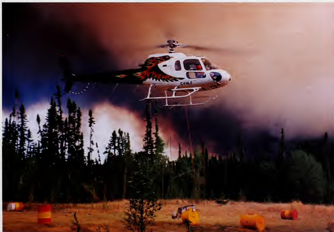
Aerospatiale twin turbine A-Star owned by Phoenix Helicopters of Fort McMurray operates helitorch for back-burning. Back-burning is a way of fighting fire with fire. This aircraft later became Air One for Edmonton Police Service
