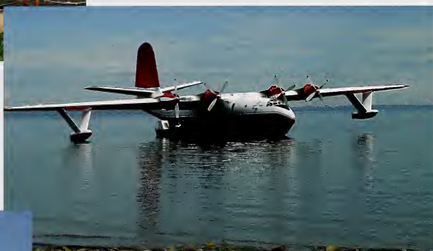
Flying Tankers Inc., Martin Mars water bomber on Slave Lake, 2002. This airtanker is capable of holding 6,000 gallons and was brought into Alberta to work on the late spring and early summer fires in Slave Lake and Lac La Biche John Brewer
