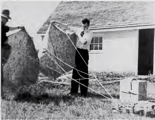
Gordon Fowlie (L) and Jack Dempsey inspecting burlap chutes used for para-cargo trials in the mid-1940s. Note equipment pack on the ground attached to the parachute
