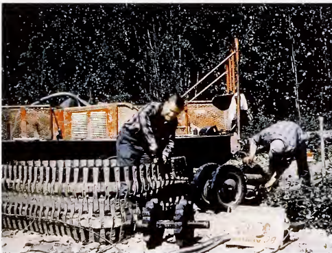
Repairing track and wheel assembly on tracked vehicle, fall, 1959, Slave Lake Forest. Doug Lyons (L) and Fermen L'Hirondelle. Lyons was the Forester-in-Charge Survey Parties Cliff Smith
