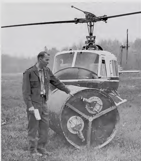
Helicopter and 300 gallon monsoon water bucket, with Fire Control Officer Bernie Simpson, Slave Lake, 1968
