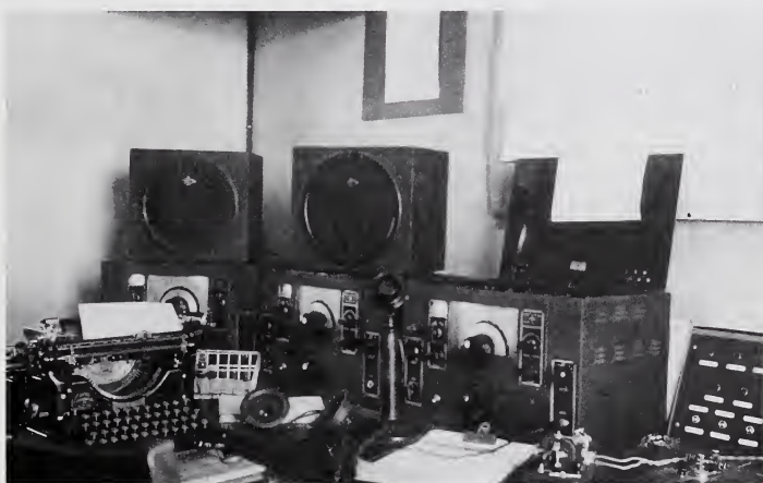
Radio dispatch centre with 3 NC 100 National Receivers, Morse Code pad and typewriter, 1940s
