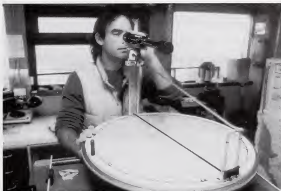
Lookout observer Bob Tough using scope and firefinder to identify location of smoke, Moose Mountain Lookout, Bow Crow Forest, 1987 Roger Meyer
