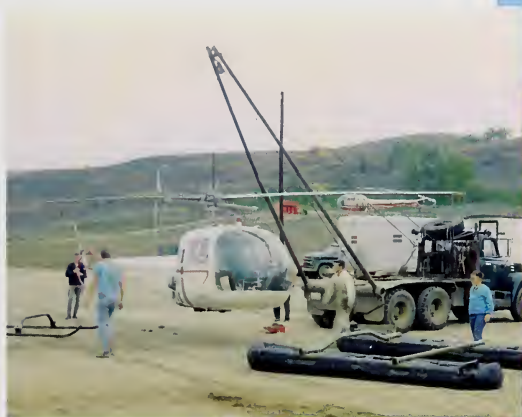
Exchanging skids for floats on a Bell 47J, mid-1960s Cliff Smith
