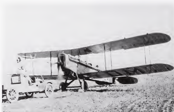
Vehicle used to crank aircraft engine, 1920s, High River, Bow River Forest
