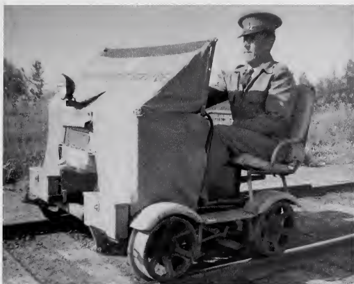
Superintendent Bert Coast uses speeder for patrol on the Northern Alberta Railway near Fort McMurray, early 1960s. Speeders were used to patrol rail lines and follow trains to detect and extinguish fires caused by cinders and sparks from steam locomotives
