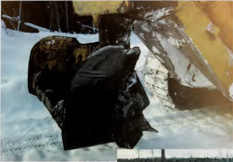
Ripper plow mounted on Caterpillar D8K preparing cutblock for planting, early 1990s Alberta Government, AFHPC
