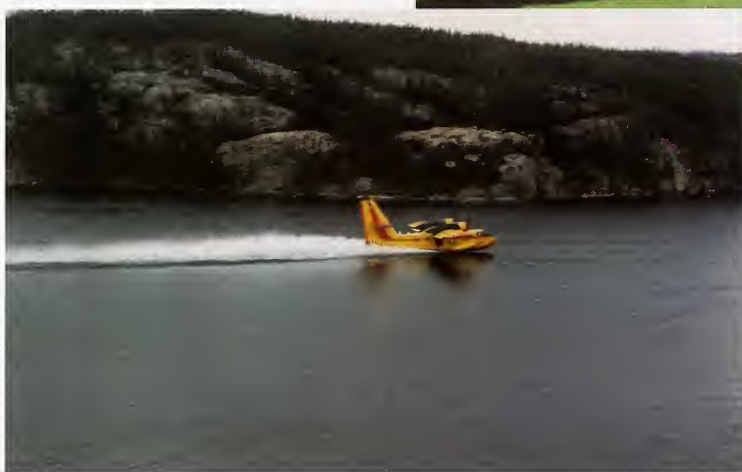
Canadair CL-215 skimming lake to pick up water load. The water is then injected with a foam concentrate before dropping on a fire. This mixture extends the effectiveness of the water and will help to 'smother' (remove the oxygen from) a surface fire if left untouched Terry Van Nest
