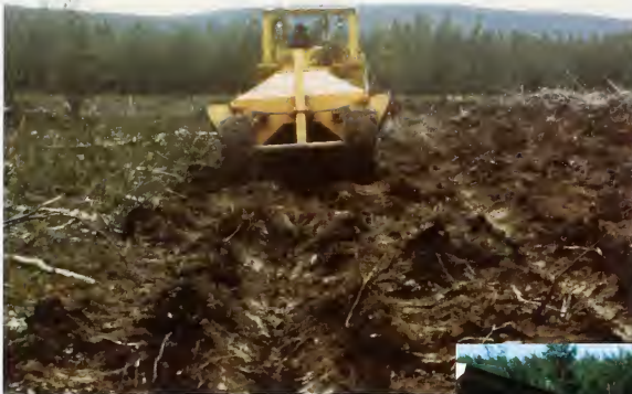
The Martinni Plow was used on sites where deep organic material existed, thus requiring a deeper 'plow' to expose mineral soil for planting Alberta Government, AFHPC
