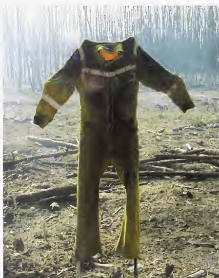
Fire resistant coveralls being tested during the ICFME test burns, Fort Providence, NWT, 1999 Gary Dakin
