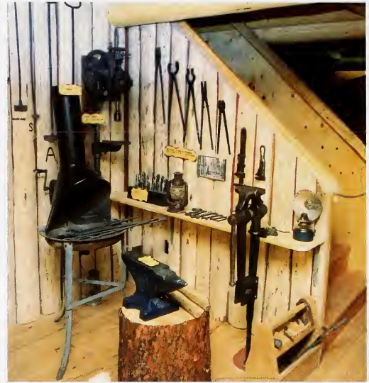
Forge and tools used for branding and shoeing horses, AFS Museum, Hinton, 1980s
