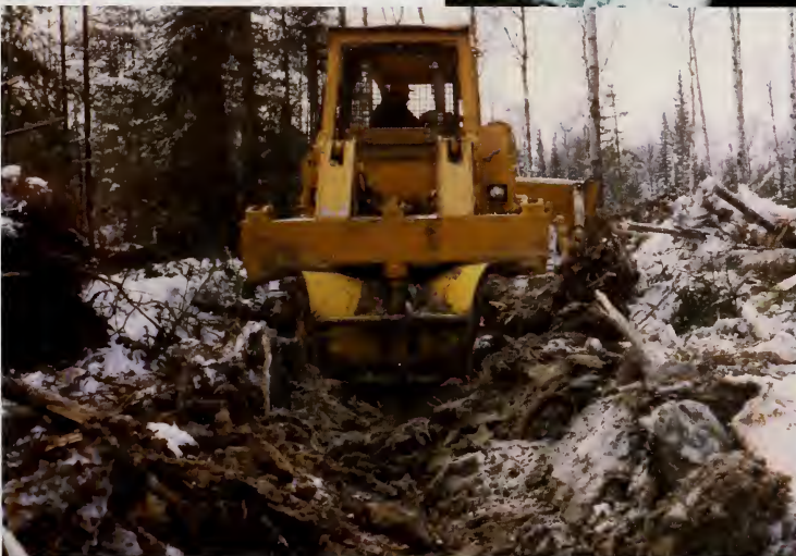
Ripper plow mounted on International HD31 preparing cutblock for planting, early 1990s Alberta Government, AFHPC
