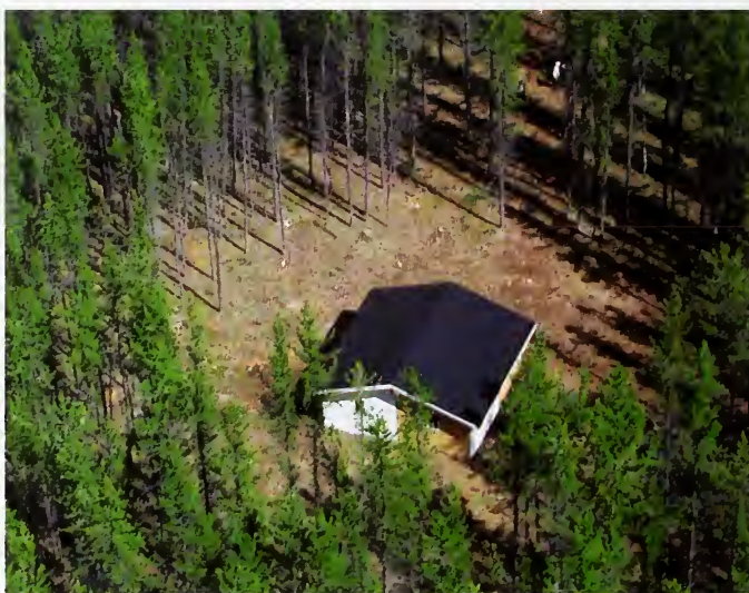
House constructed within one of the ICFME test plots to study the effects of radiant heat on structures and the fuel-free zone required for structures to survive wildfires in a forested setting, Fort Providence, NWT, 1998 Gary Dakin
