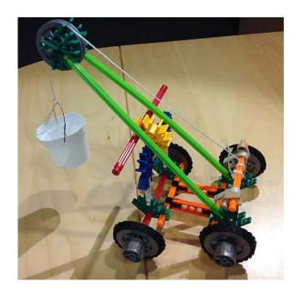
This design of an excavator has four wheels attached to two axles for moving, and it has a pulley-and-bucket system for moving dirt.
