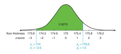
0.62% of the flooring has thickness less than 174 mm 93.32% of the flooring has thickness less than 175.6 mm 93.32% -0.62% = 92.7%
