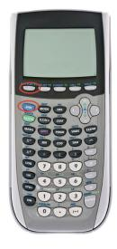
To see a graph of the plotted points, press the  $2^{nd}$  button, and then the STAT PLOT button.
