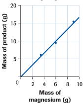
Figure 3 The relationship between the mass of magnesium that reacted and the mass of product obtained is a straight line (direct proportion).
