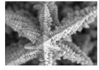
Figure 1 Image of a silver crystal taken with a scanning electron microscope (SEM).
