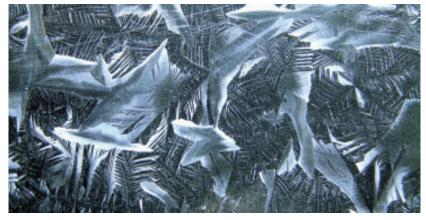
The crystal structure of metals normally can be seen only under a microscope. On the surface of zinc-plated (galvanized) objects, however, large flat crystals of zinc are plainly visible.
