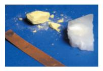
Figure 1 Different solids-copper, sulfur, and paraffin wax-behave very differently under mechanical stress.
