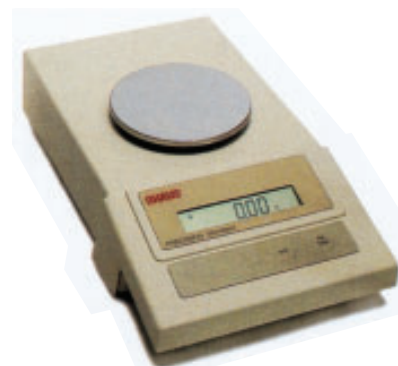
Figure 1 An electronic balance is simpler to operate and more efficient than the older mechanical balance. Electronic balances also provide the convenience of taring (Appendix C.3).
