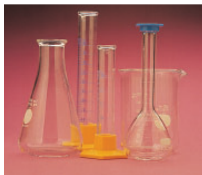
Figure 2 Volumetric glassware comes in a variety of shapes and sizes. The Erlenmeyer flask on the far left has only approximate volume markings, as does the beaker. The graduated cylinders have much better precision, but for high precision, a volumetric flask (on the right) is used. The volumetric flask shown here, when filled to the line, contains 100.0 mL \pm 0.16 mL at 20 °C. This means that a volume measured in this flask is uncertain by less than 0.2 mL at the specified temperature.
